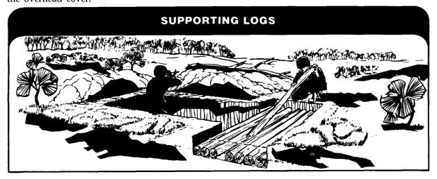
Then put 15 to 20 cm (6 to 8 in) of dirt on top of the waterproofing material. Cover the dirt with the sod and camouflage it.
