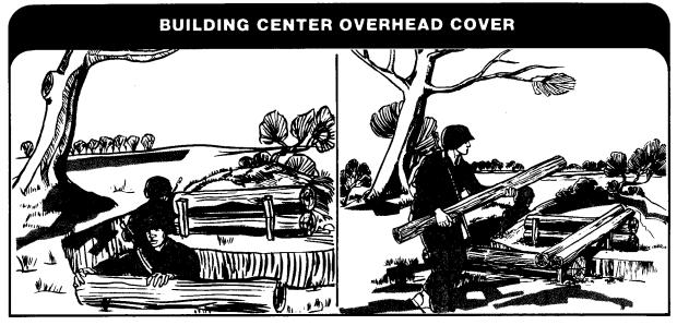
Put a water-repellent layer, such as C-ration boxes or a poncho, over the base logs.
