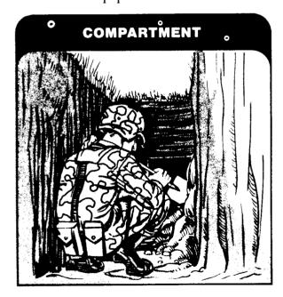
In sandy or loose soil, the sides of your position may require **revetments** to keep them from collapsing. Use such things as mesh wire, boards, or logs for revetting. Tie anchor string, rope, or wire to the revetting material and stake them down. Drive the stakes into the ground. This hides them and keeps them from being mistaken for aiming stakes or sector stakes.
